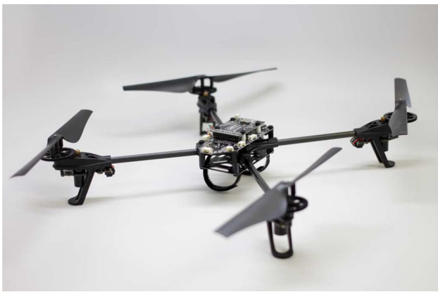
Fig. 10 The quadrotor used in the experiments consists of a PX4 IMU with an AR. Drone frame and motors
