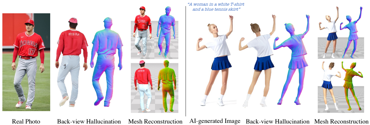
Figure 1. Single-view textured human reconstruction. SiTH is a novel pipeline for creating high-quality and fully textured 3D human meshes from single images. We first hallucinate back-view appearances through an image-conditioned diffusion model, followed by the reconstruction of full-body textured meshes using both the front and back-view images. Our pipeline enables the creation of lifelike and diverse 3D humans from unseen photos ( left ) and AI-generated images ( right ).
