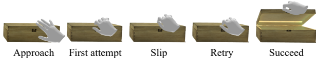
Figure 4. Qualitative articulation result. The hand shows some recovery ability from failure cases. Zoom in for details.
