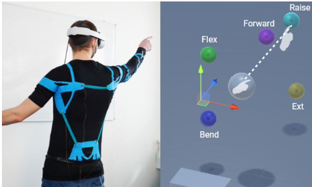
Figure 10: User study setup. Participant wearing Auto-Designed garment and reaching for target (left), and their corresponding motion in the virtual environment (right).
