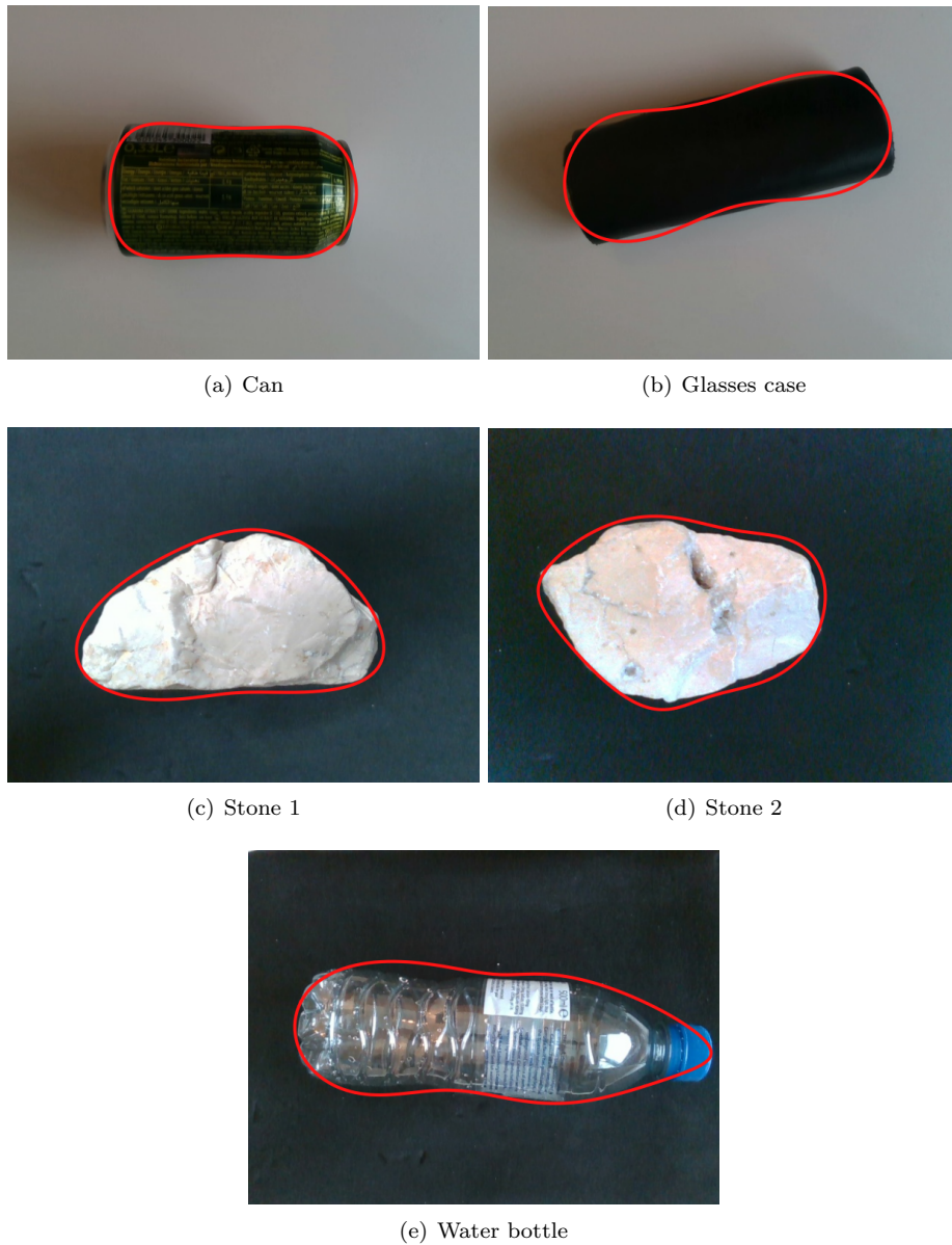
Figure 4.7: EFD contours with 4 harmonics for the test objects
