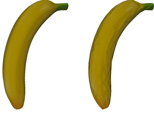
Figure 6. Mesh Decimation. We use mesh decimation to reduce the number of vertices of the object mesh. On the left is the original object mesh, on the right the decimated mesh. This helps to speed up the physics simulation during training.
