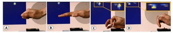
Figure 2. Signal properties. Pixel intensity corresponds to reflected energy; horizontal axis is velocity; vertical axis is range. (A+B) Sensor produces almost identical response for static objects even of distinct shape. (C+D) In contrast, the sensor resolves even minute motion with high resolution.
