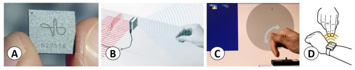
Figure 1. We explore interactive possibilities enabled by Google's project Soli (A), a solid-state short-range radar, capturing energy reflected of hands and other objects (B). The signal is unique in that it resolves motion in the millimeter range but does not directly capture shape (C). We propose a novel gesture recognition algorithm specifically designed to recognize subtle, low-effort gestures based on the Soli signal.
