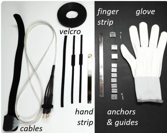
**Figure 4.** Assembly of the ES brake, 3D printed guides and attachments fastened to thin nylon glove using velcro.
