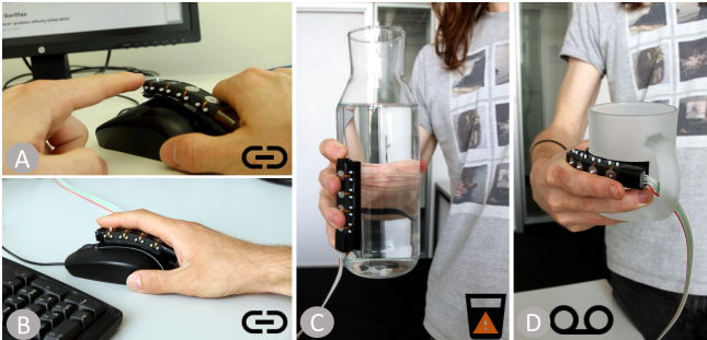
Figure 7. MagTics can be used to augment existing objects and input devices. A–B): A standard mouse gets augmented with output capabilities to enhance desktop productivity. C–D): Everyday objects, such as water bottles and coffee mugs, turn into notification proxies.
