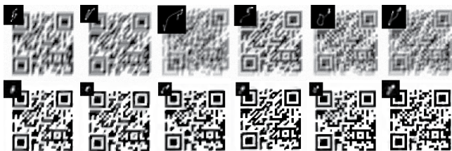
Figure 4: Removing synthetic uniform blurs. Top: input images and ground truth kernels. Bottom: output images and kernel estimates when first decoded. Kernel size indicates the scale level.
