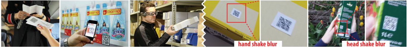
Figure 1: Left three: Scanning visual codes with handheld and wearable devices is becoming ubiquitous. Right four: When the camera or the scanned object move even slightly during scanning, the captured visual codes become distorted by motion blur and conventional decoder algorithms cannot decode them.
