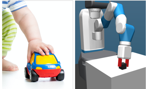
Fig. 1. Inspiration of our work comes from intrinsic motivation of infants exploring the world through physical interactions. We model tactile sensing with force sensors (red) and leverage tactile information to accelerate learning.
