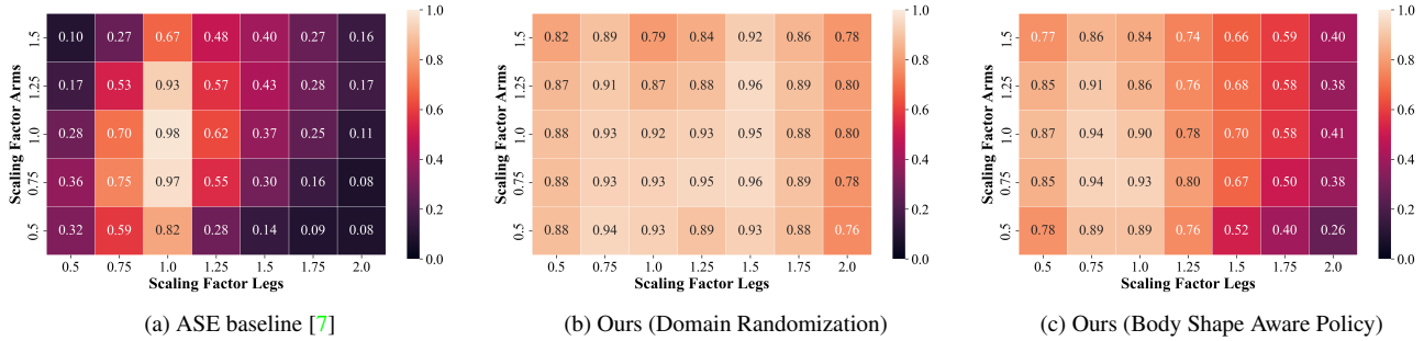
Figure 2. Evaluation. Average success rates across varying body shapes, displayed as heat maps for the baseline [7] and our two approaches. Our method can better adapt to varying body shapes, which is indicated by the higher success rates (brighter colors).
